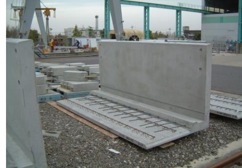
Half Precast Slab (Balcony)
